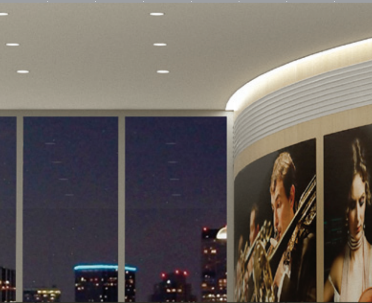
Theater Atrium / Lobby Lumen packages used: 2500 and 3000 Beam angles used: 40°
