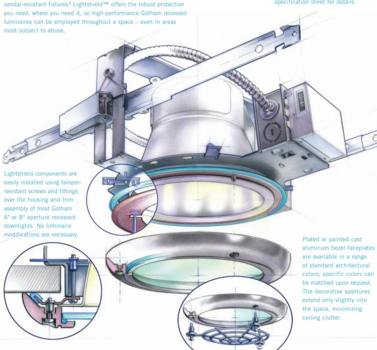
Protected by Lightshield, Gotham recessed luminaires assure comfortable, low-brightness illumination in high-abuse areas. Patented Bounding Ray™ reflectors optimize efficiency and optical control of all available lamping sources – compact fluorescent, metal halide or incandescent.
